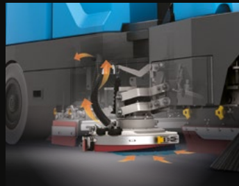
Side scrubbing brush with vacuum system
