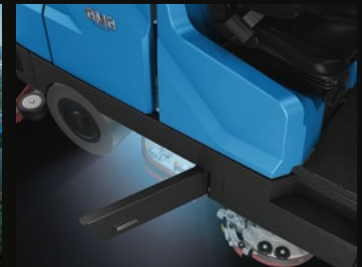
Service LED lights
